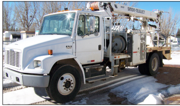
2001 - Freightliner chassis with a 1995 Terex digger derrick
