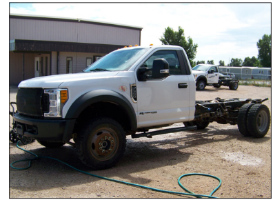
Unit 4017: 2017 Ford F-550; 6.7L V8 diesel engine; 4x4 automatic, single cab; 112,119 miles
