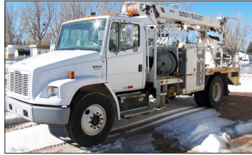
2001 - Freightliner chassis with a 1995 Terex digger derrick
