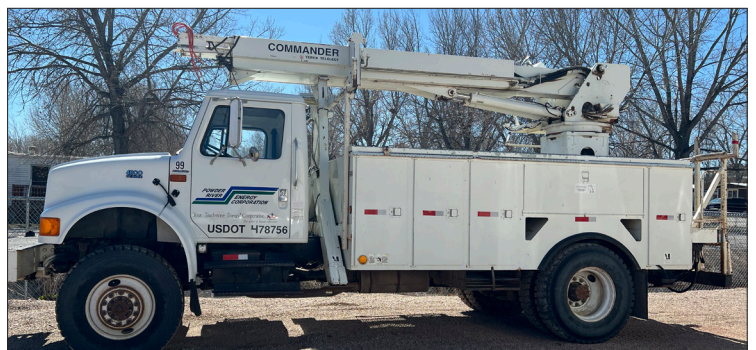
2001 International 4x4 4800 series dt466 diesel; Manual trans, boom is inop. Good service body.
